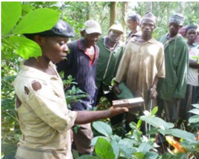
Canopy cover measurement using a spherical densitometer by a VNRC member from Mkanga 1 village, Lindi.
