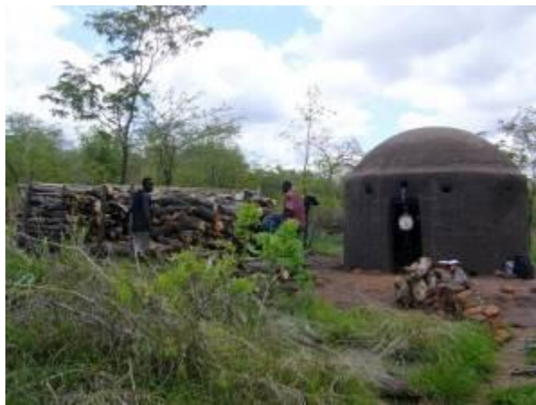
Figure 12: Dar Charcoal “Half-Orange” Kiln – Rufiji, Tanzania
