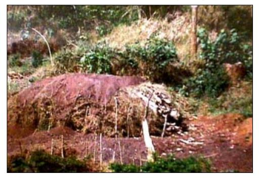
Figure 1 Typical charcoal kiln under preparation at Kitulangalo area.
