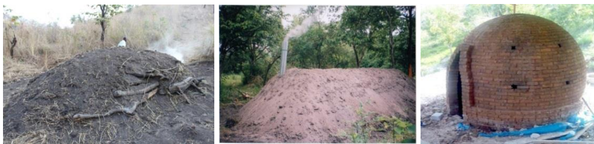
Figure 21: Charcoal kilns compared in this study: basic earth mound kiln (BEK), improved earth mound kiln (IBEK) and half-orange brick kiln (BK) (source: TaTEDO)
