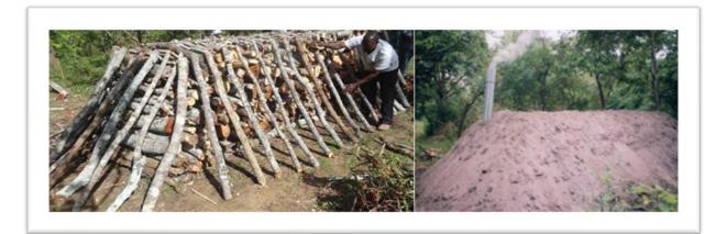
Figure 19: Improved earth mound kiln (IEMK) for charcoal production in Kilosa<sup>54</sup>
